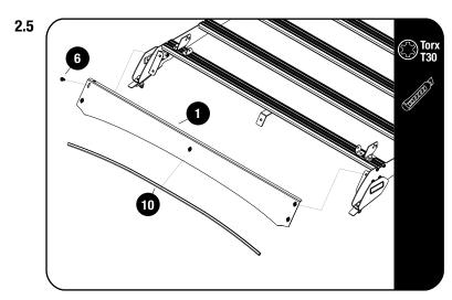
Fit the Wind Fairing Rubber (Item 10) to the Light Bar Wind Fairing (Item`1). Using the notched section as a guide, trim if needed.
