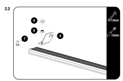
Fit the Light Bar Bracket 01 LH / RH (Item 4) for for the 40" Light Bar, using M8 x 16 Hex Bolt & M8 Nyloc Nut (Items 7 & 9). Fit the light bar and center it on the slat before fully tightening the brackets.
