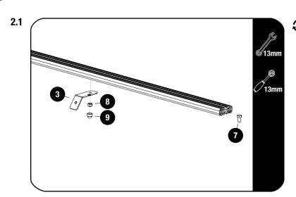
Slide one M8 x 16 Hex Head Bolt (Item 7) into the T-slot of the front slat. Center the mid support bracket (Item 3) in the middle of the slat and secure using M8 Nyloc Nut (Item 8). Loosly assembly.
